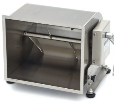
Stainless steel housing, mixing wing and lid
