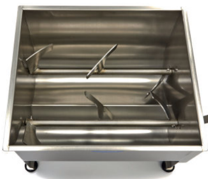
Stainless steel housing, mixing wing and lid
