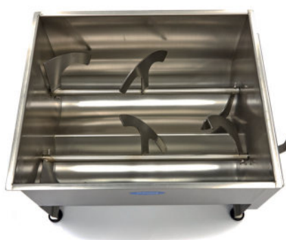
Stainless steel housing, mixing wing and lid
