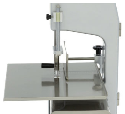
Spacious table with calibration plate
